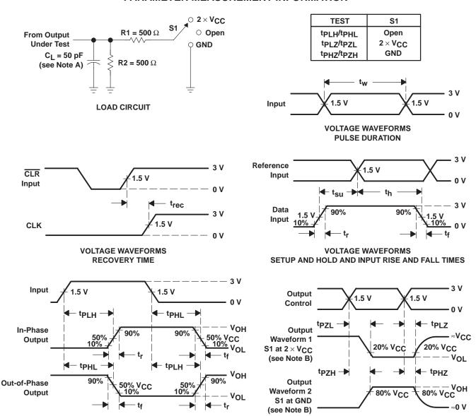
NOTES: A. C<sub>L</sub> includes probe and test-fixture capacitance.
